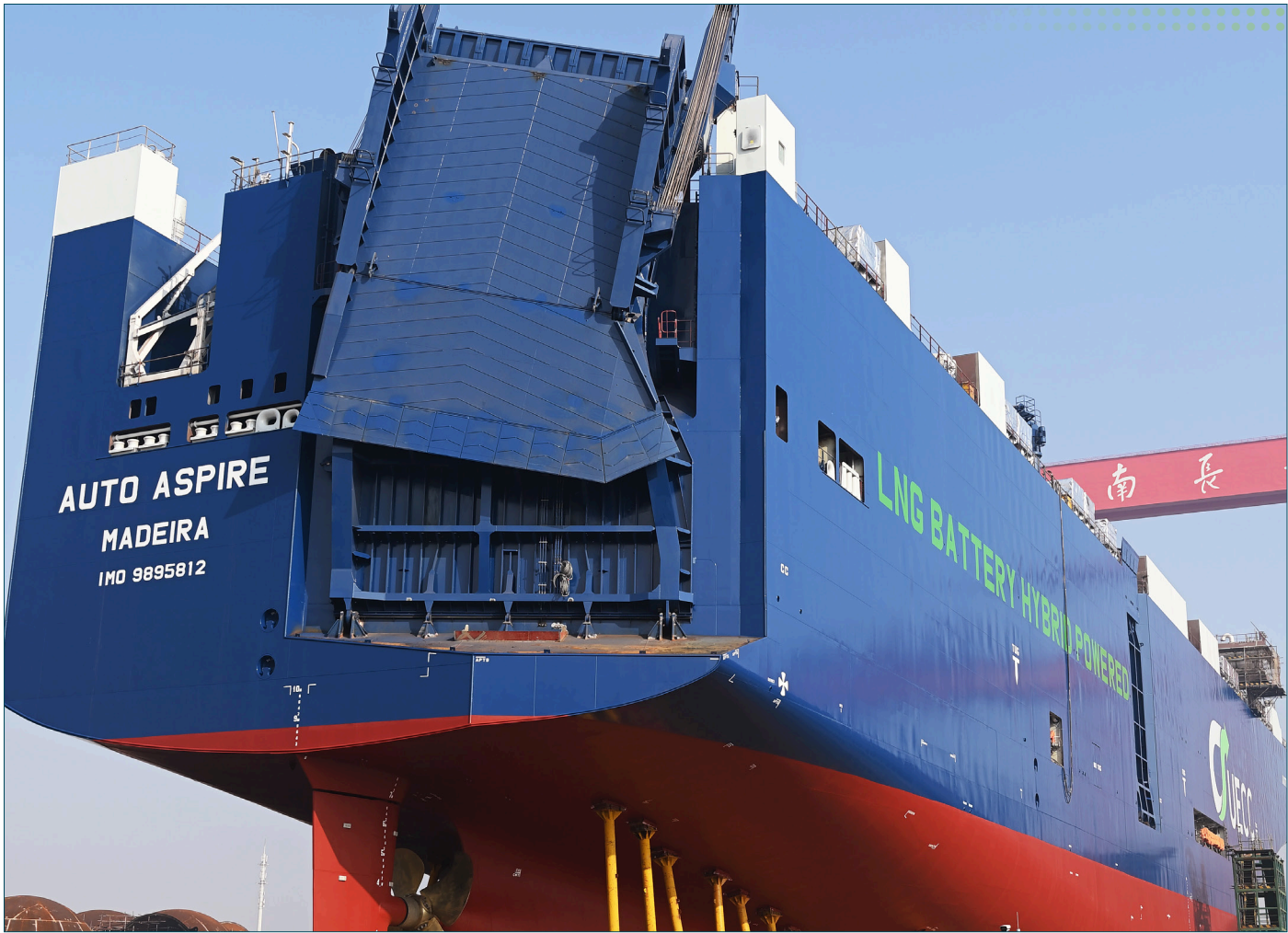
New breed: newbuild Auto Aspire, one of three of the world's first multi-fuel LNG battery hybrid PCTCs earlier ordered by UECC, is shown before being launched at China' Jiangnan Shipyard in early 2022
